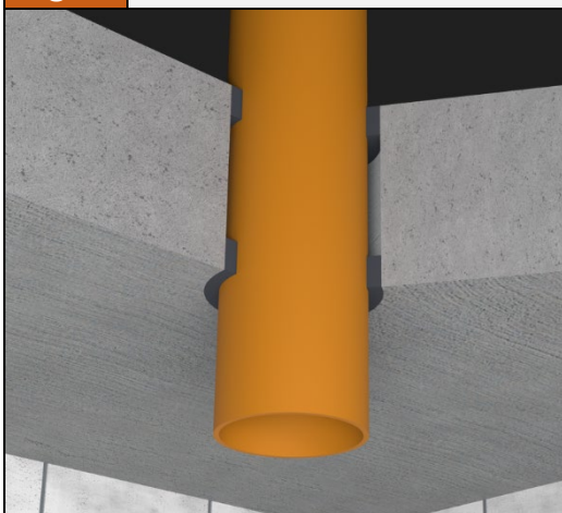
Fig.7 Combustible pipes penetration seals in rigid floor with thickness A \geq 150 mm and density \rho \geq 550 kg/m 3
