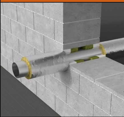
Fig. 1 Penetration seal in wall A \geq 150 mm
