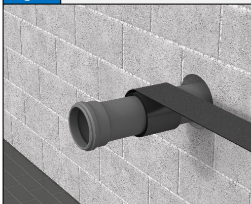
Fig.1 Combustible pipes in a flexible or rigid wall with a thickness of A ≥ 150 mm
